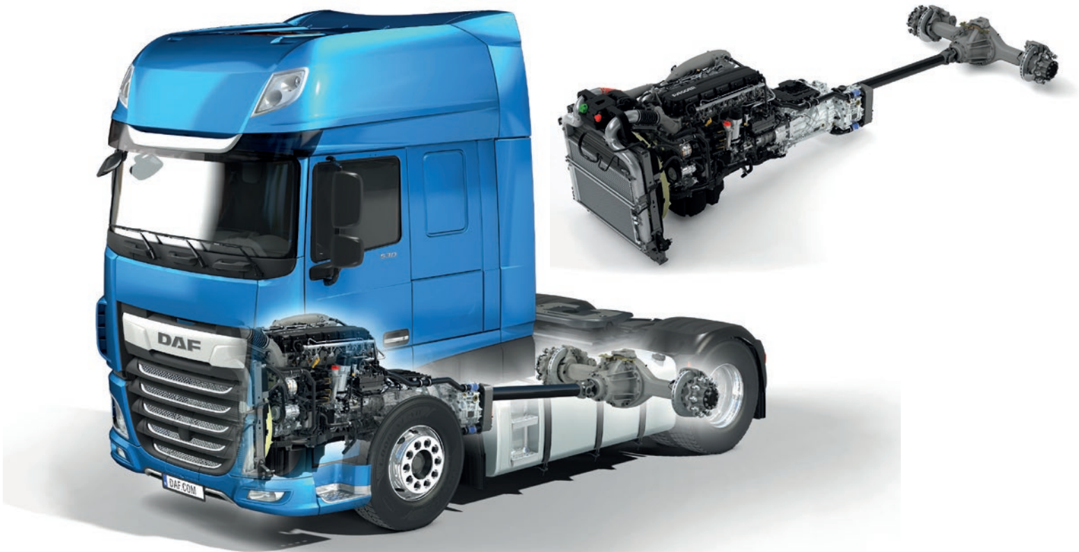
Top: The MX-13 engine boasts a range-topping 530hp and an extra 100Nm of torque
